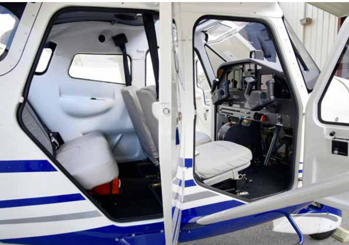
**PUSHRODS** actuate the stabilator and rudder on the Vulcanair V1.0, a four-seater designed to stand up to the rigors of landings at unimproved airstrips. A third door means rear-seat passengers can enter on the co-pilot's side without disturbing front-seat occupants. Thoughtful touches on the Italian trainer include locking and covered fuel caps to keep water from seeping into the fuel tanks (see facing page).
