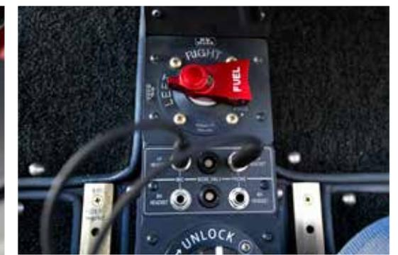
**GARMIN G500** primary and multifunction displays, digital backup instruments, and a JPI engine monitor give students the technology they've come to expect in the digital age. Just a little movement of the large trim wheel on the power quadrant keeps the trainer trimmed in all phases of flight, and a machined fuel-tank selector is positioned in the center of the floorboard alongside headset jacks, a parking brake, and USB ports.
