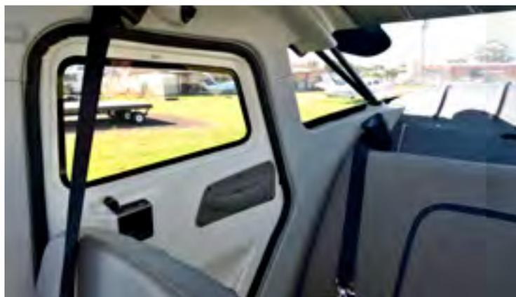
Leaving the external inspection behind, entry to the aircraft is easy via a single step attached to the airframe just below the door sill. Visible airframe 'down tubes' extend vertically at each corner of the cabin. At the front, these are reminiscent of an Auster or a Piper Cub but are offset well to the side to not impede the forward vision. However, they are very convenient handholds for climbing aboard or when adjusting the seat position.
